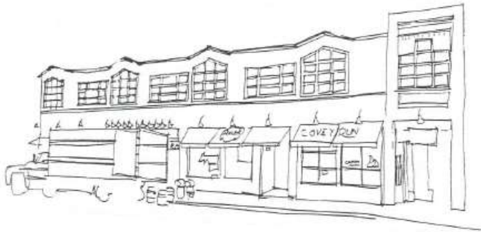
9 10 Figure IV.C.1.(c). The roofline, windows, and details of these examples are coordinated to provide a 11 rhythmic breakup of an otherwise horizontal building. Note how the awnings and lights provide 12 human scale while their repetition relates back to the building massing. 13 14
