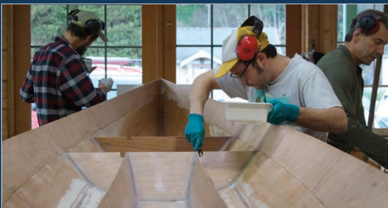
Student Kendra (K) Woolfe works on fitting the white oak breast hook on the Port Hadlock Work Skiff.
