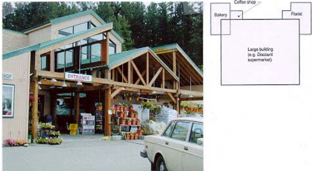
Figure IV.C.1.(a). Clustering smaller activities around the entrance to a large building adds human scale and minimizes the large building bulk. The Thriftway Market effectively incorporates this concept, adding human scale and visual interest to its entrance.
