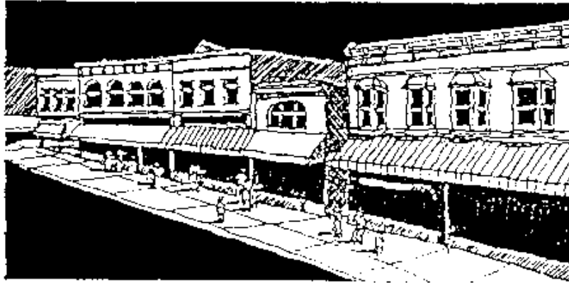
Align the bottom edge of awnings, canopies or marquees on a group of buildings so that the unity of the store front line is maintained with adjacent buildings.
