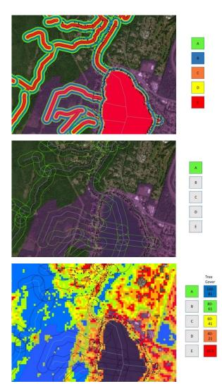
Figure \_\_\_. Options for evaluating attributes within a buffered stream centerline.
