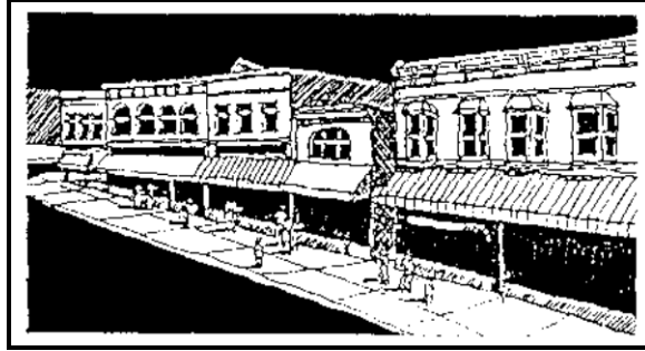
Align the bottom edge of awnings, canopies or marquees on a group of buildings so that the unity of the store front line is maintained with adjacent buildings.
