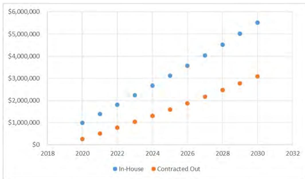
**Figure 7–3. CIPP project lifetime costs assuming 1,500 LF of replacement per year with 2.5% inflation**
