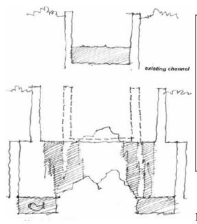
Strawberry Creek Slough Diagram illustrates a horizontal expansion of the creek channel (with optional cascade storage pools) to spread and slow the flow of water, establish new habitat, and increase visual open space for the community. Improved security and safety fencing design improves the appearance of the creek corridor while maintaining safety.
