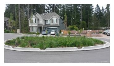
Bioretention BMP in a cul-de-sac of a LID residential neighborhood in construction in western WA. The bioretention manages stormwater runoff from the roadway and contributing roof and driveway areas. Numerous large existing trees were retained, adding valuable stormwater and community benefits.
